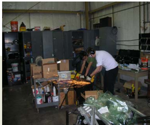
Top: Chassis team members cut chromoly steel pipes. Right: Members applying epoxy to build one of the trailer shelves.
