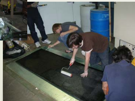
Top: Chassis team members cut chromoly steel pipes. Right: Members applying epoxy to build one of the trailer shelves.
